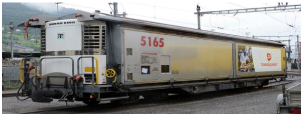
Haikq-qy 5165 TransGourmet, Kühlag. Neu
